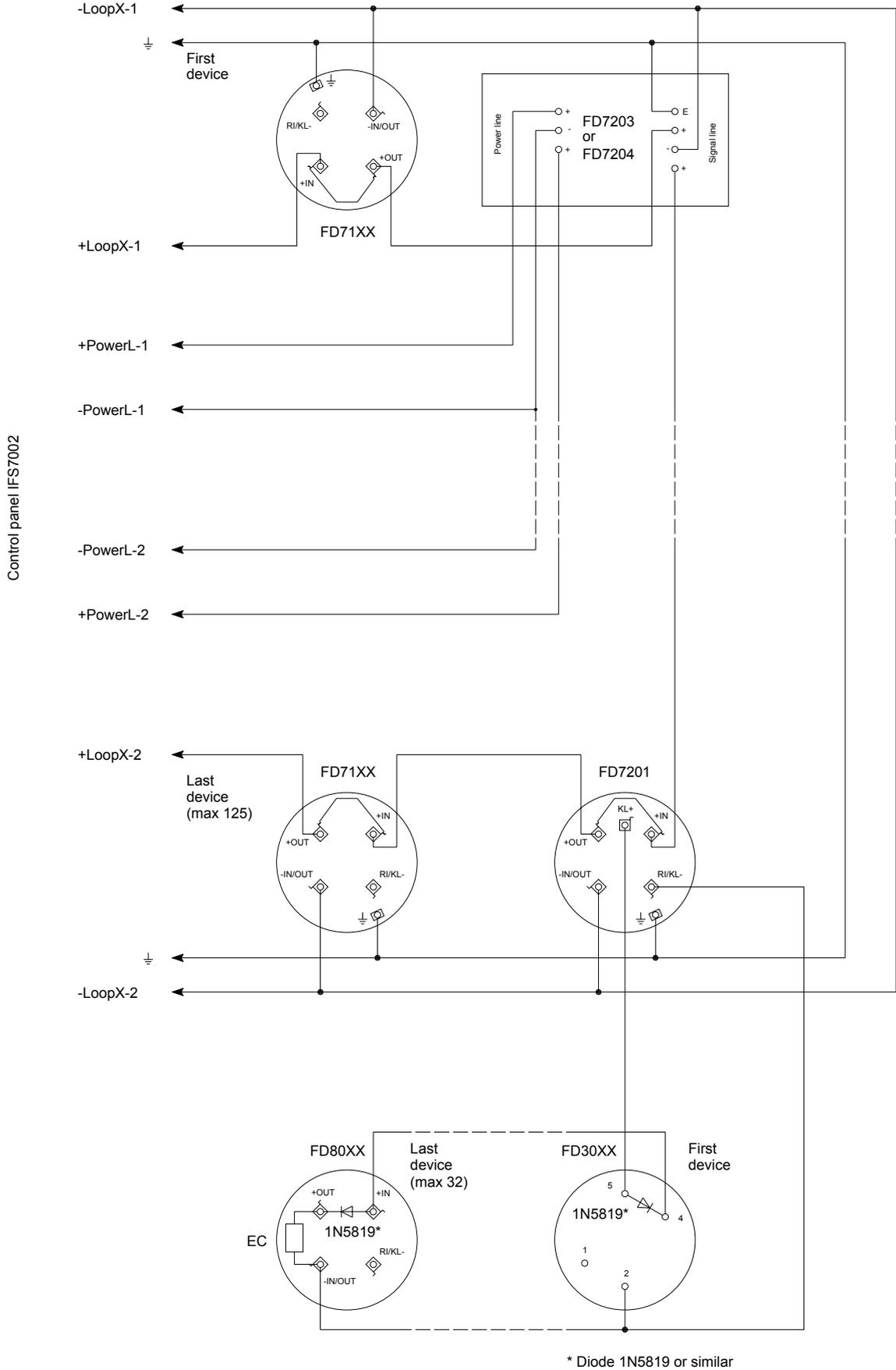
a) Connection of addressable devices to fire alarm loop and power loop
