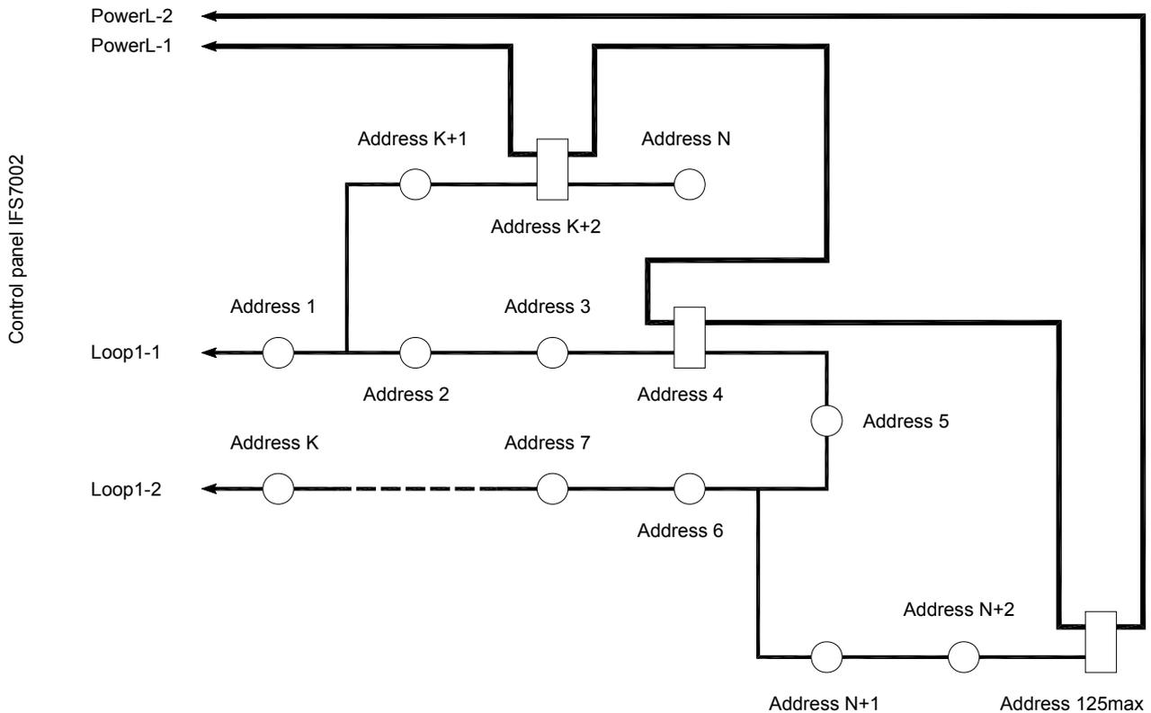
c) Configuration of Fire Alarm Loop with branches and Power Loop (proper connection)
