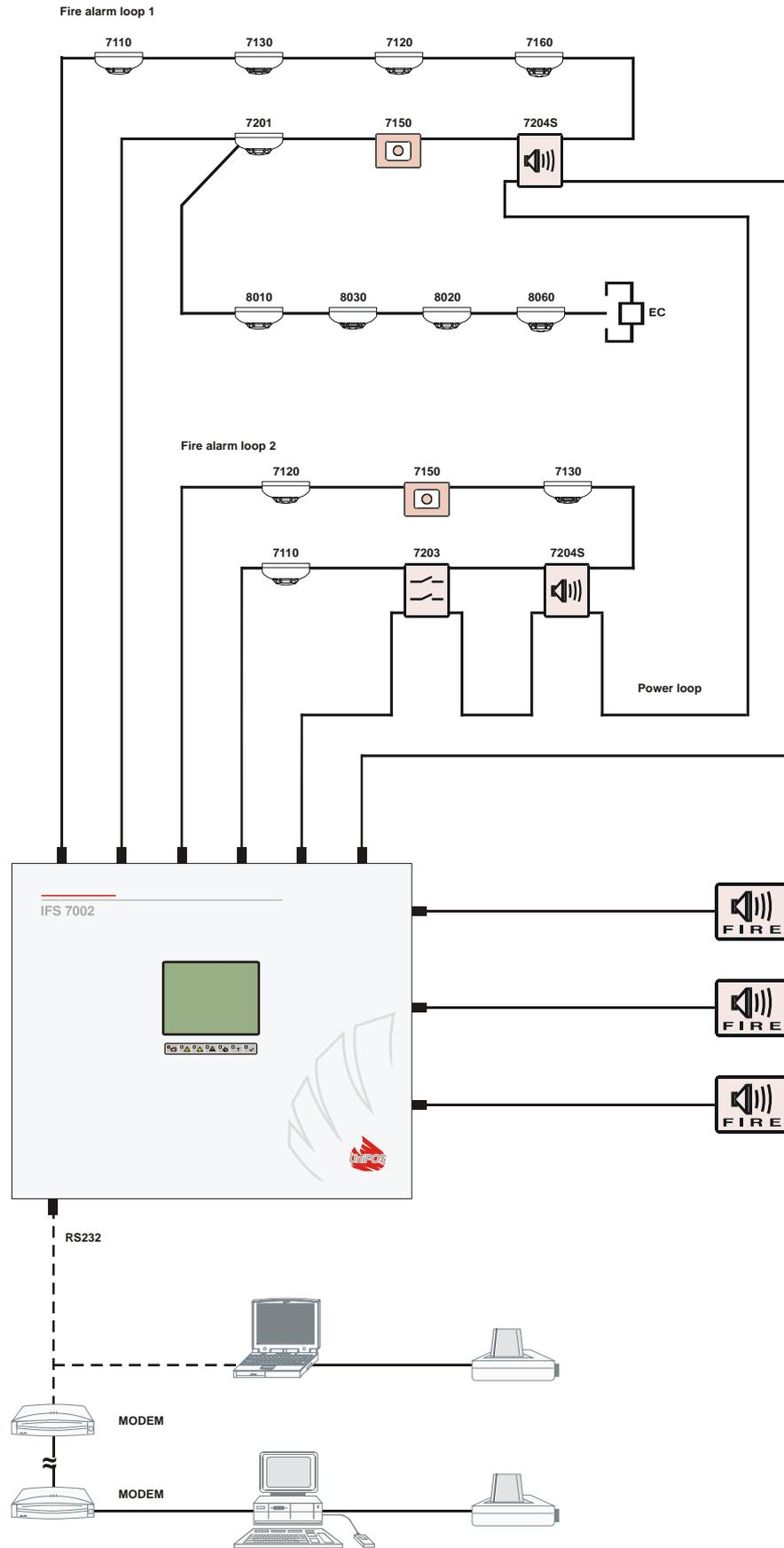
Block diagram of fire alarm installation designed on the base of IFS7002
