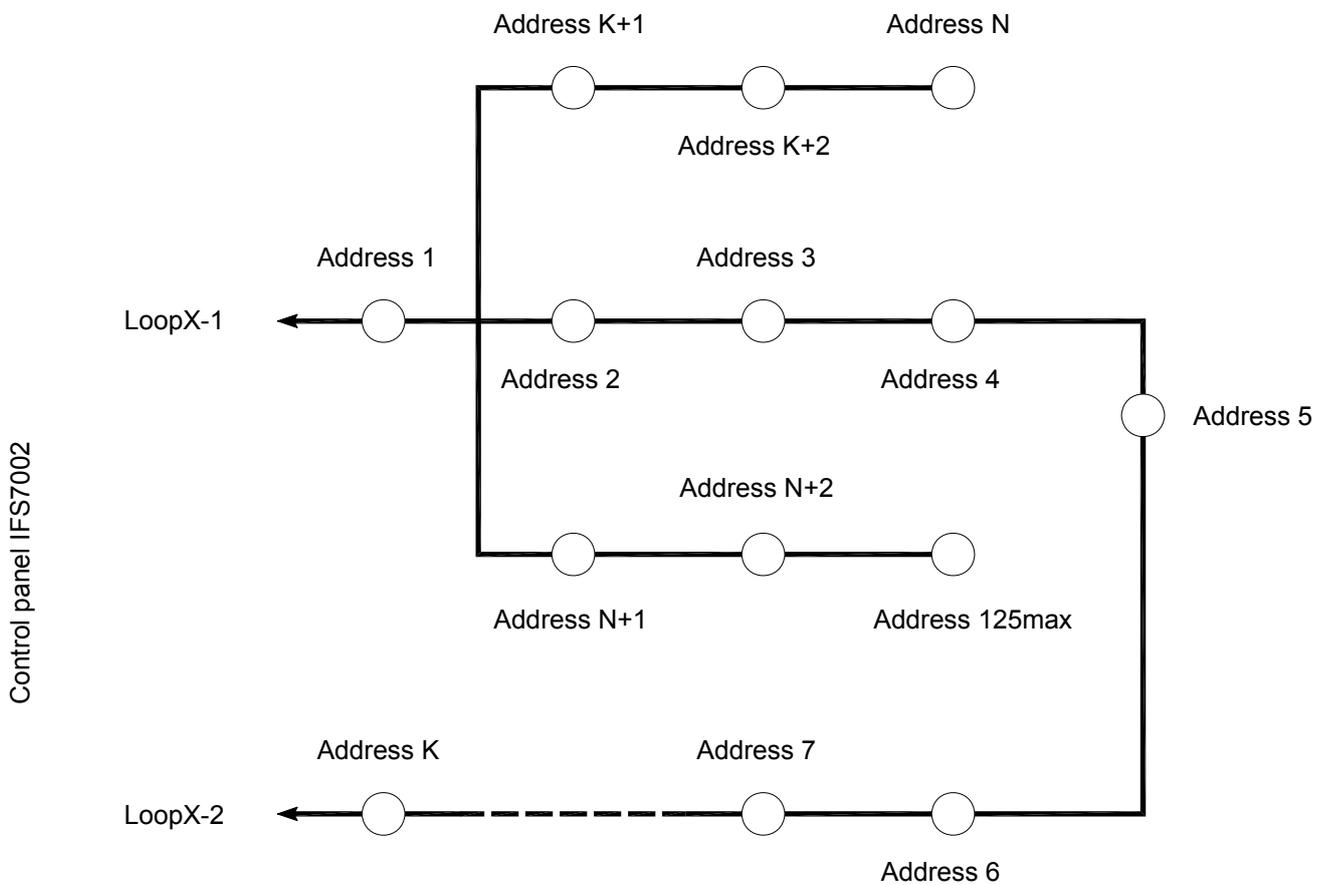
e) Improper connection of Fire alarm loop branches
