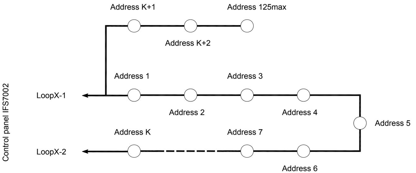
d) Improper connection of Fire alarm loop branch
